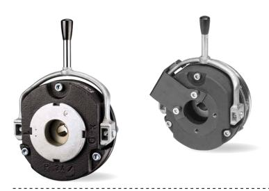
On our spring-applied/spring-loaded brakes from the BFK458 series, the HFC friction lining (HFC stands for "high friction coefficient") allows us to increase the braking torque by around 20% without any change in size. Thus, by choosing a spring-applied brake with an HFC friction lining, you can save valuable installation space and cut costs.
