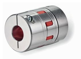
The ROTEX<sup>®</sup> GS is a three-piece coupling that can be plugged in axially and is backlash-free under initial tension. It impresses even in critical applications thanks to its backlash-free torque transmission, rigidity that matches the individual deployment and excellent vibration damping. This coupling is particularly easy to mount and provides the user with production-optimised installation options.
