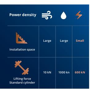
Pneumatic cylinders are limited by the maximum pressure and energy losses due to air compression. Large cylinder diameters and high pressure levels are required to generate high forces. Electromechanical cylinders offer a **higher power density** and require **less installation space** than hydraulic cylinders, which take up more space due to pipes and hoses.
