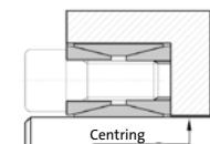
Hydraulic locking bushes are double-walled steel sleeves that contain a hydraulic medium. Pressure is exerted on the medium by tightening the pressure screw(s). This results in a uniform expansion of the steel sleeve against the shaft and hub. This results in a frictionally engaged shaft/hub connection.
