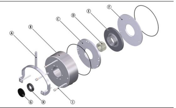
Fig. 21: Spring-applied brake INTORQ BFK470-06 to 18
