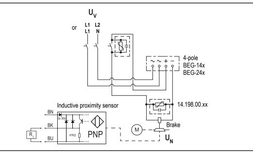
Fig. 17: Supply: Phase-phase or phase-N via 6-pole rectifier
