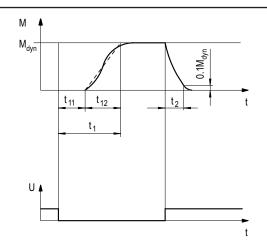
Fig. 2: Operating/switching times of the spring-applied brakes
