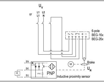
Fig. 18: Supply: Phase-phase or phase-N via 4-pole rectifier
