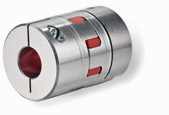
The ROTEX® GS is a three-piece coupling that can be plugged in axially and is backlash-free under initial tension. It impresses even in critical applications thanks to its backlash-free torque transmission, rigidity that matches the individual deployment and excellent vibration damping. This coupling is particularly easy to mount and provides the user with production-optimised installation options.
