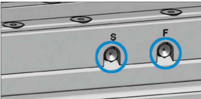
Figure 1.12 ___ Slider unit with laterally placed grease nipples
